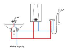
N.B. Instantaneous water heating is the most energy efficient way of directly heating water electrically, however, the delivered water temperature will be dependent upon the incoming water temperature, supply voltage and selected flow rate.
